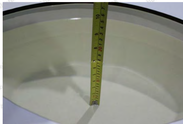
Liquid depth in the body phantom (5GHz)
