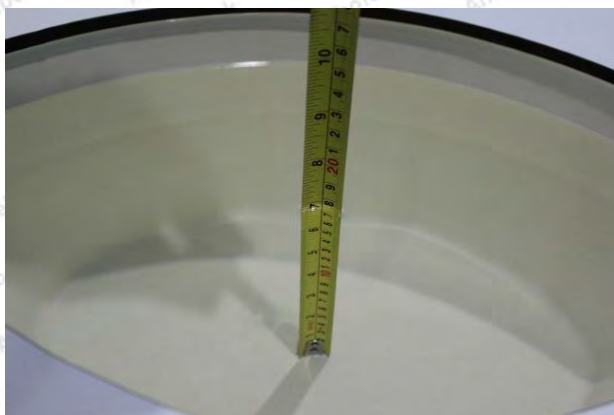
Liquid depth in the body phantom (5GHz)
