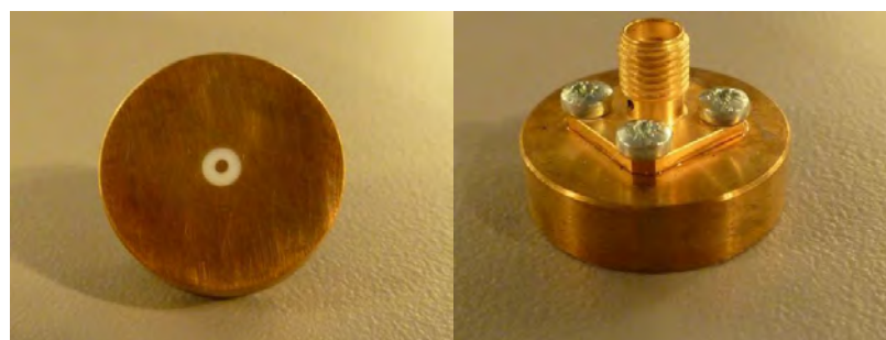
Figure 1 – MVG LIMESAR Dielectric Probe
