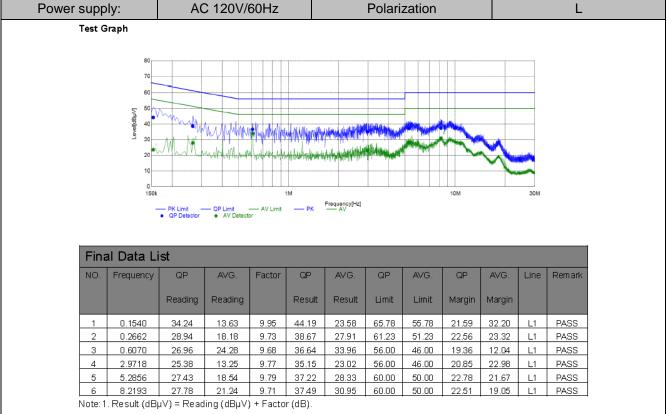
2. Factor (dB) = Cable loss (dB) + LISN Factor (dB).
