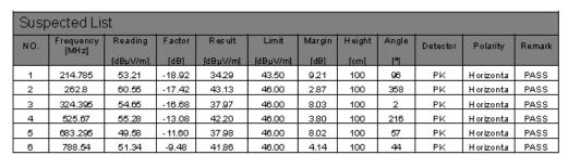
Note:1. Result (dB $\mu$ V/m) = Reading(dB $\mu$ V/m) + Factor (dB).
