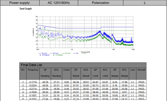
Note: 1. Result (dB $\mu$ V) = Reading (dB $\mu$ V) + Factor (dB).
