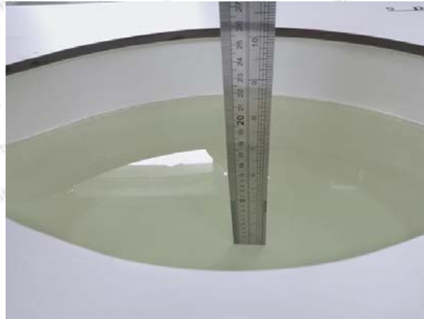
Liquid depth in the body phantom (2450MHz)
