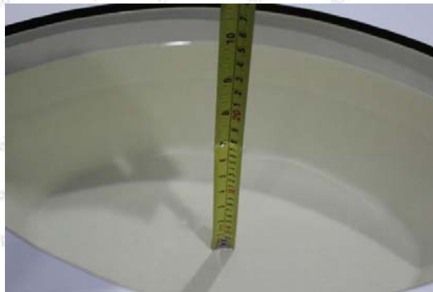
Liquid depth in the body phantom (5GHz)
