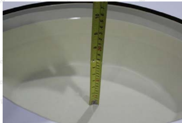
Liquid depth in the body phantom (5GHz)
