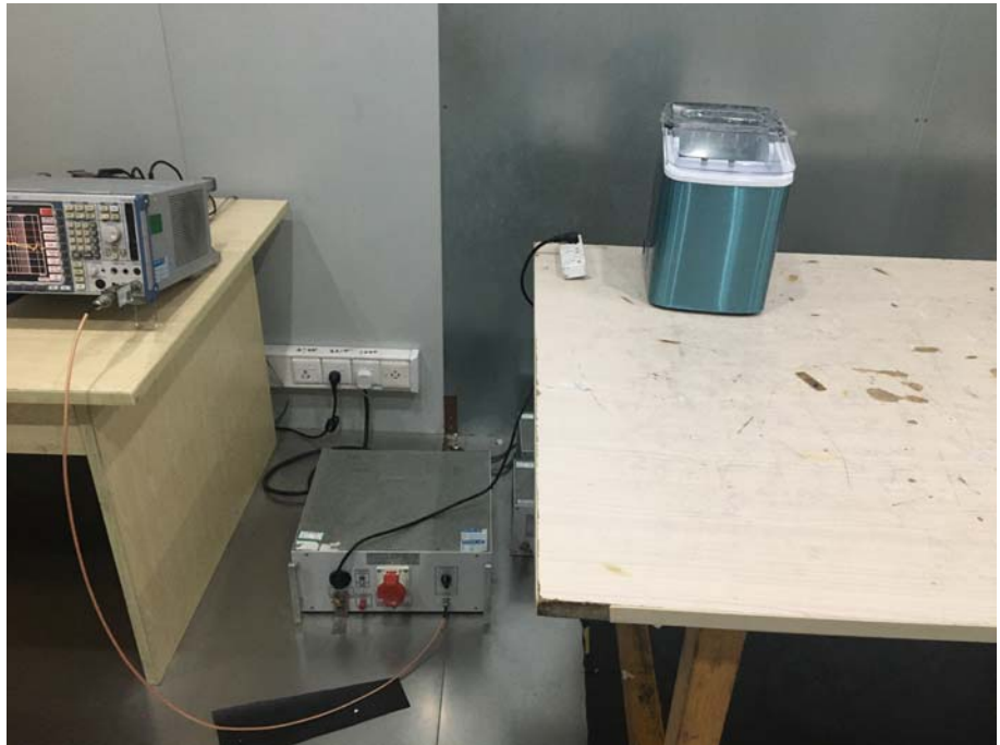
Conducted Emission Test Setup
