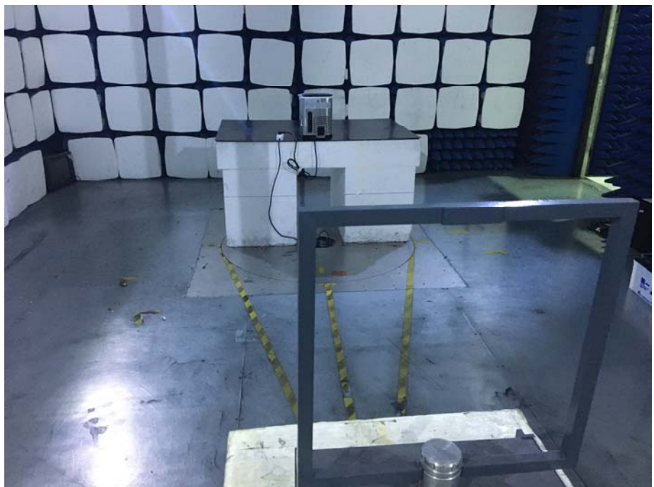
Radiation Emission Test Setup (Below 30MHz)
