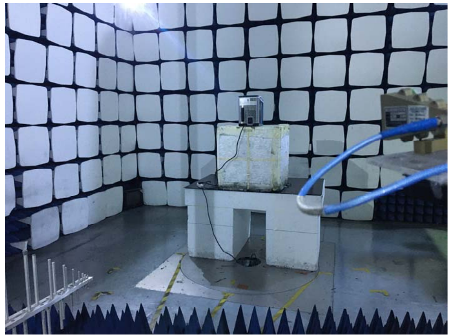
Radiation Emission Test Setup (Above 18GHz)
