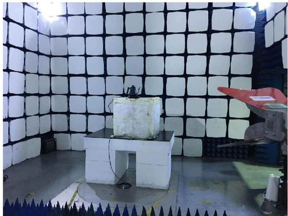
Radiation Emission Test Setup (1GHz to 18GHz)
