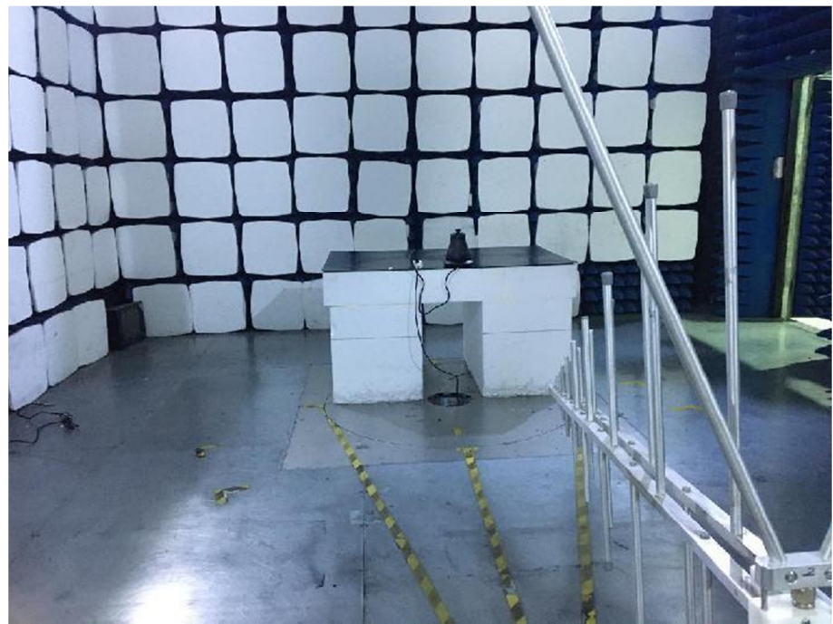
Radiation Emission Test Setup (30MHz to 1GHz)
