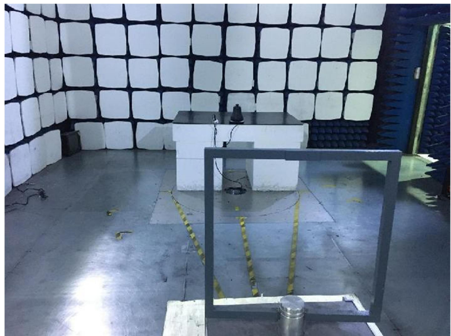
Radiation Emission Test Setup (Below 30MHz)
