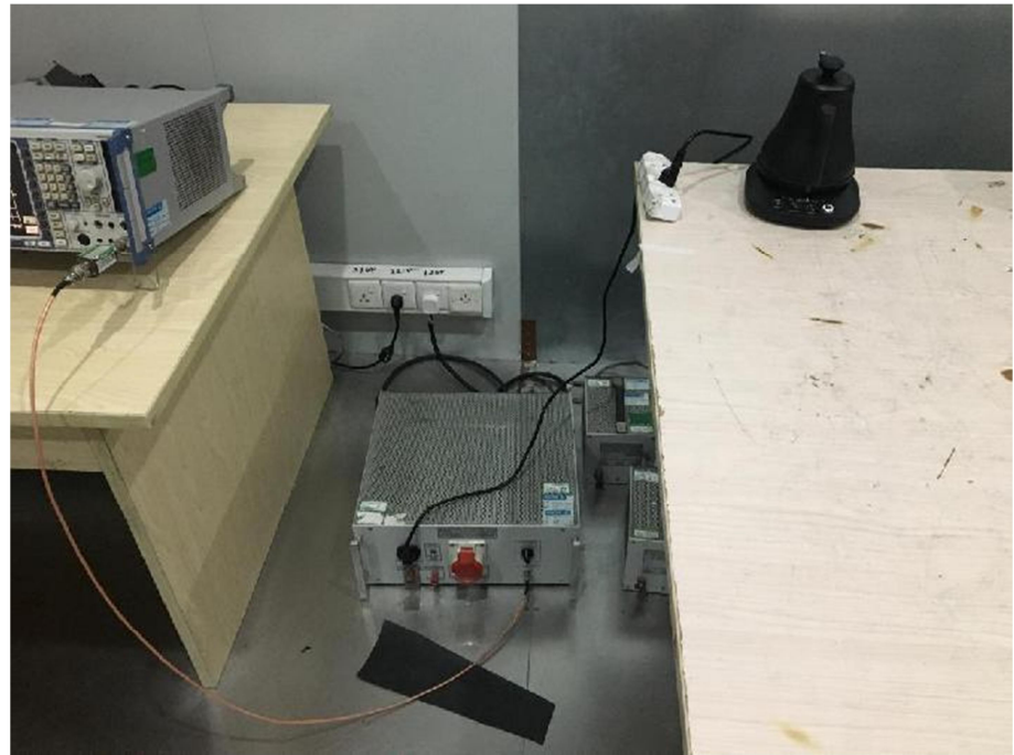
Conducted Emission Test Setup
