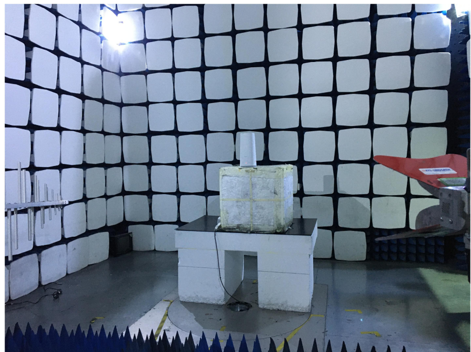
Radiation Emission Test Setup (1GHz to 18GHz)
