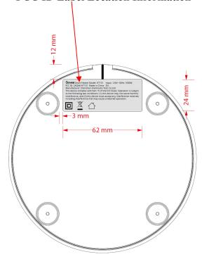
The label shown shall be permanently affixed at a conspicuous location on the device and be readily visible to the user at the time purchase (Labeling requirements per 2.925)
