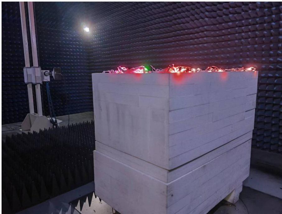
Photo of Radiated Emission Measurement (Above 1G)
