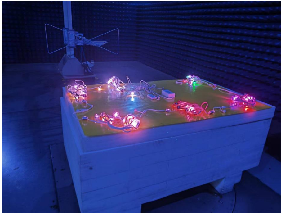
Photo of Radiated Emission Measurement (Above 1G)
