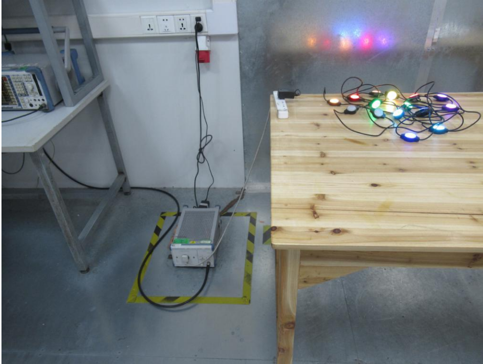
Photo of Conducted Emission Measurement
