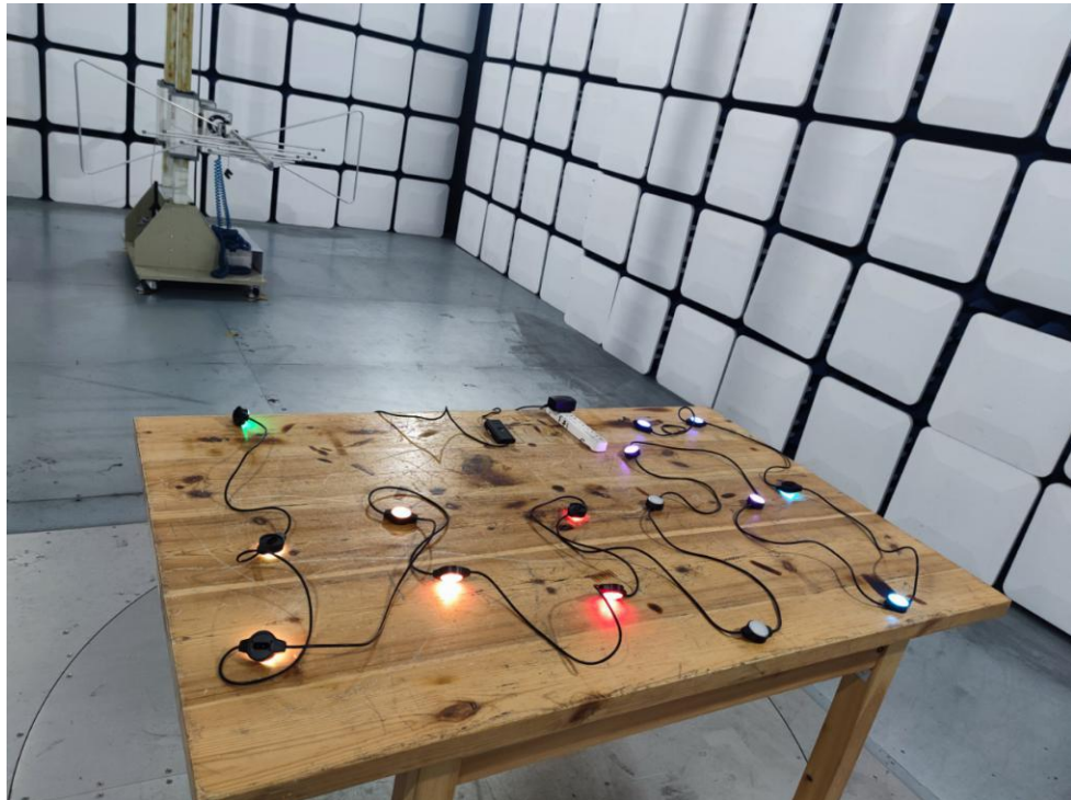
Photo of Radiation Emission Test
