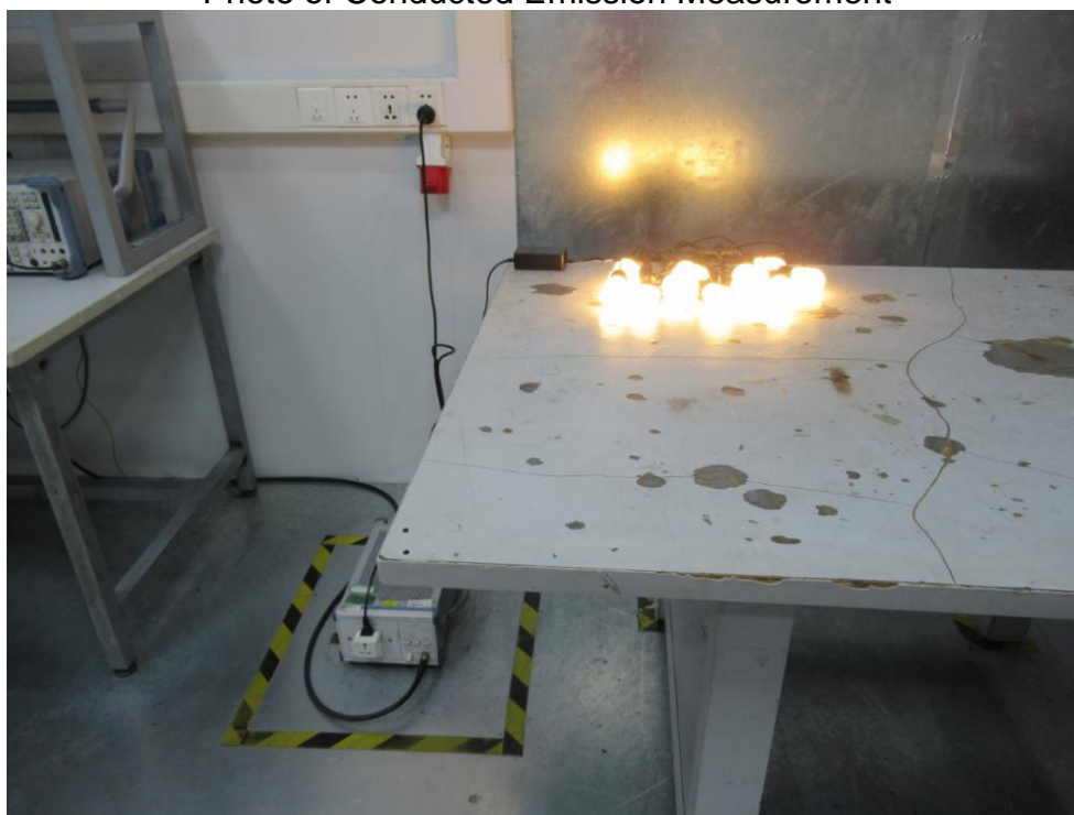
FCC ID: 2AQA6-H7001 Photo of Conducted Emission Measurement
