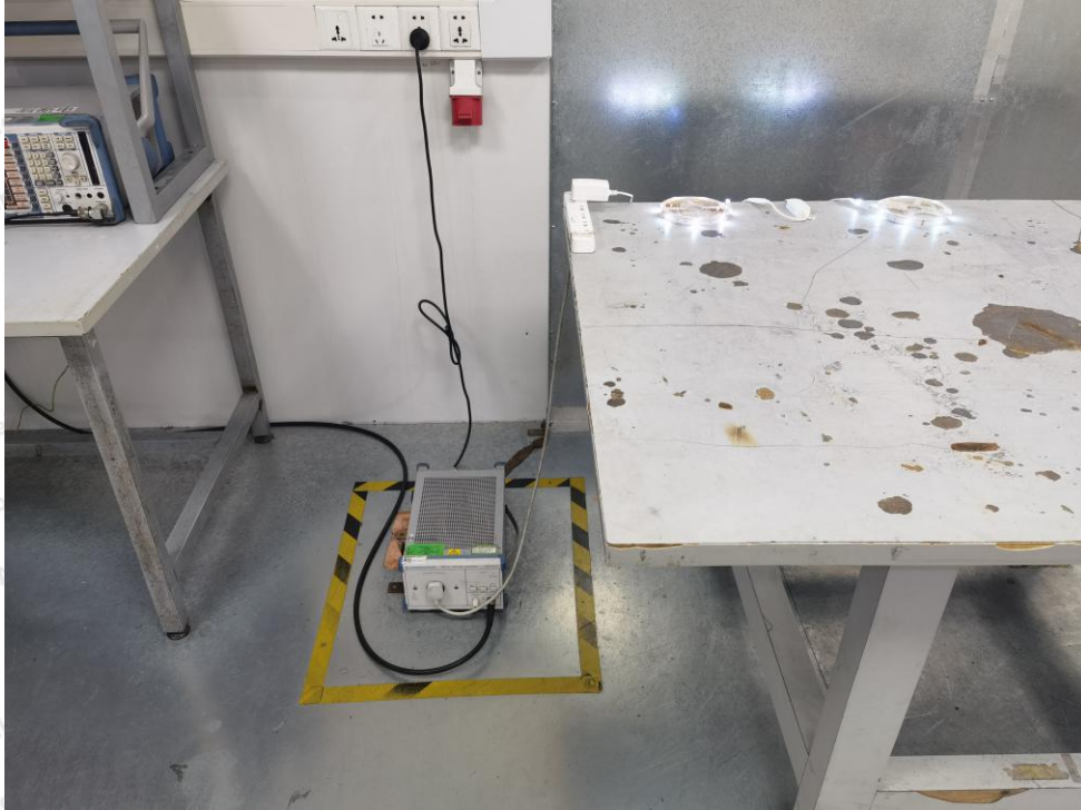
Photo of Power Line Conducted Emission Test
