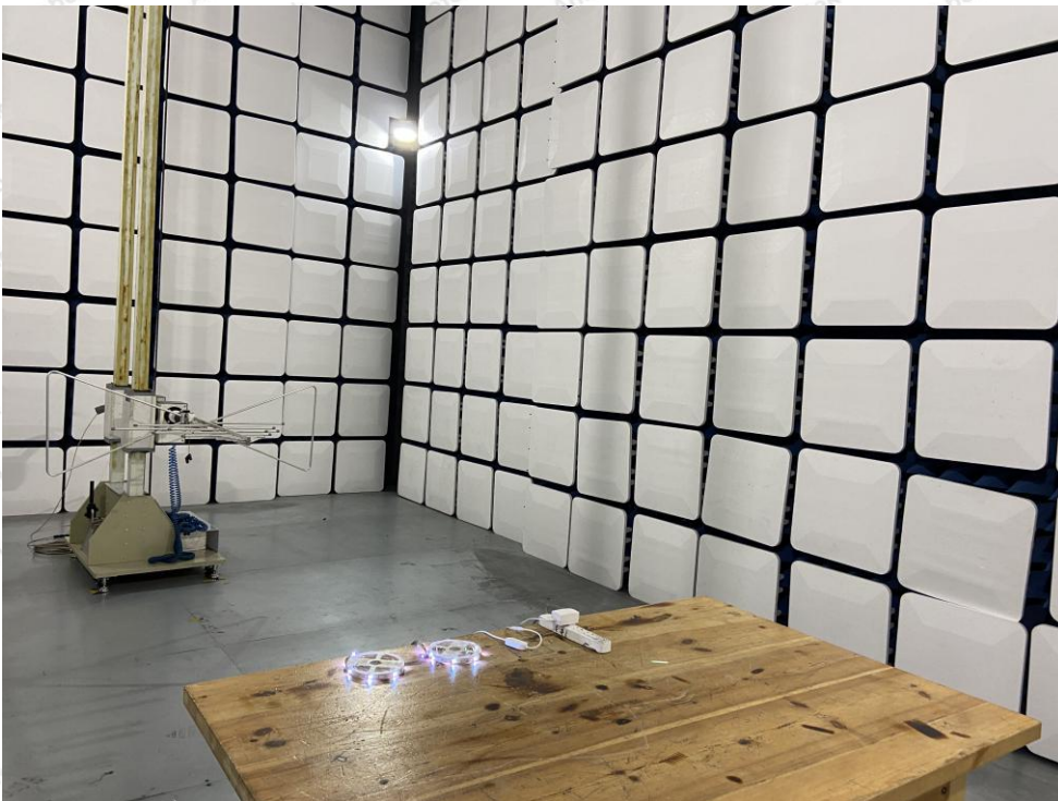
Photo of Radiation Emission Test
