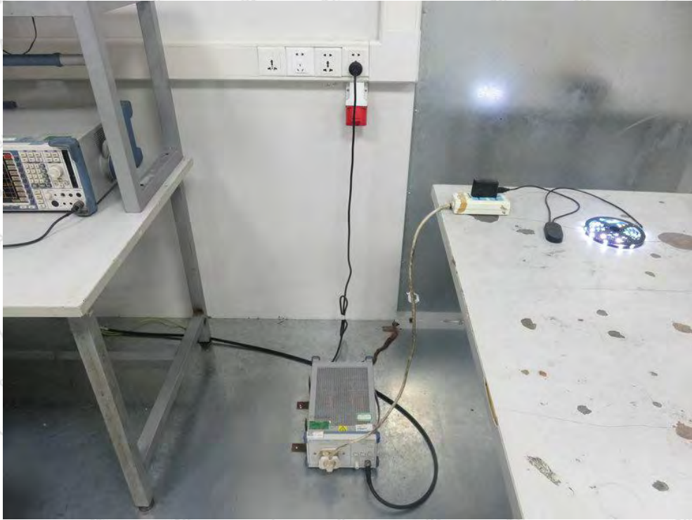
Photo of Power Line Conducted Emission Test
