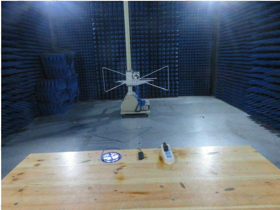
Photo of Radiation Emission Test
