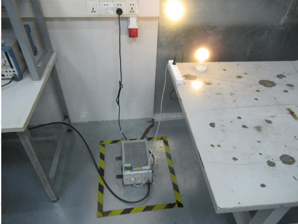
Photo of Power Line Conducted Emission Test
