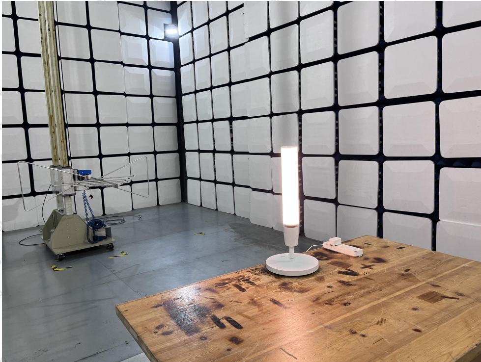
Photo of Radiation Emission Test
