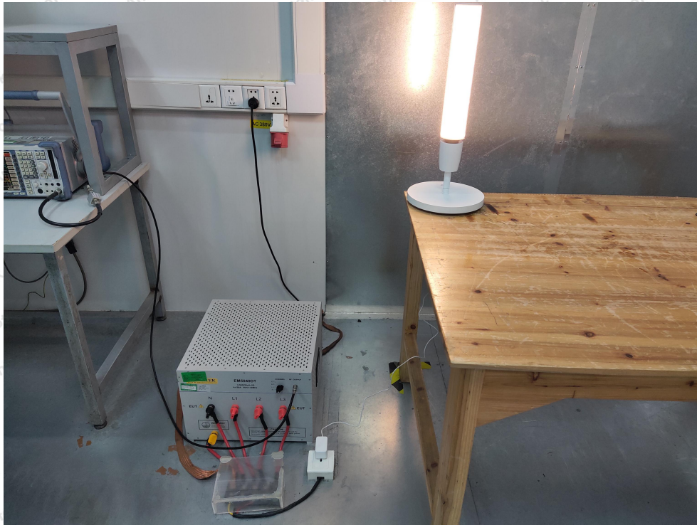
Photo of Conducted Emission Measurement
