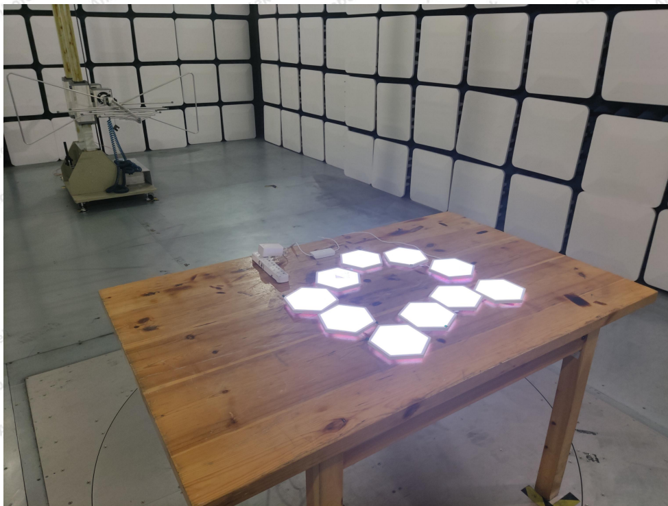
Photo of Radiation Emission Test
