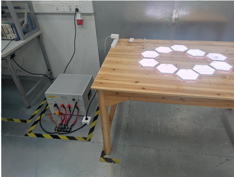
Photo of Conducted Emission Measurement
