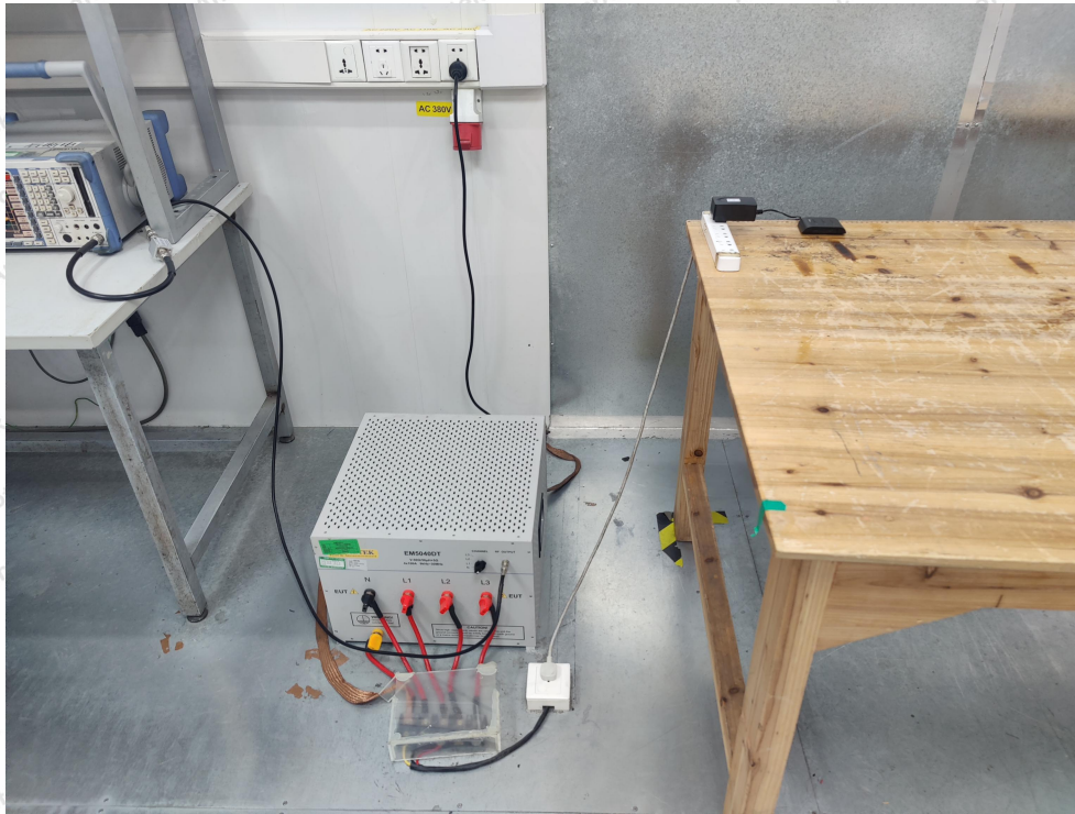
Photo of Conducted Emission Measurement
