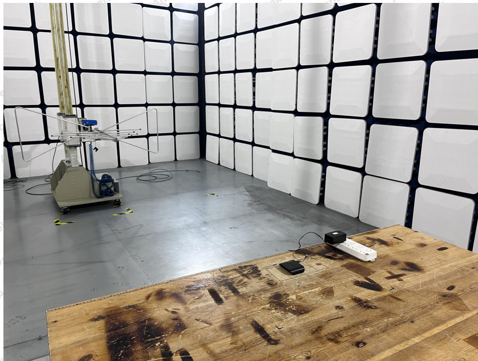
Photo of Radiation Emission Test
