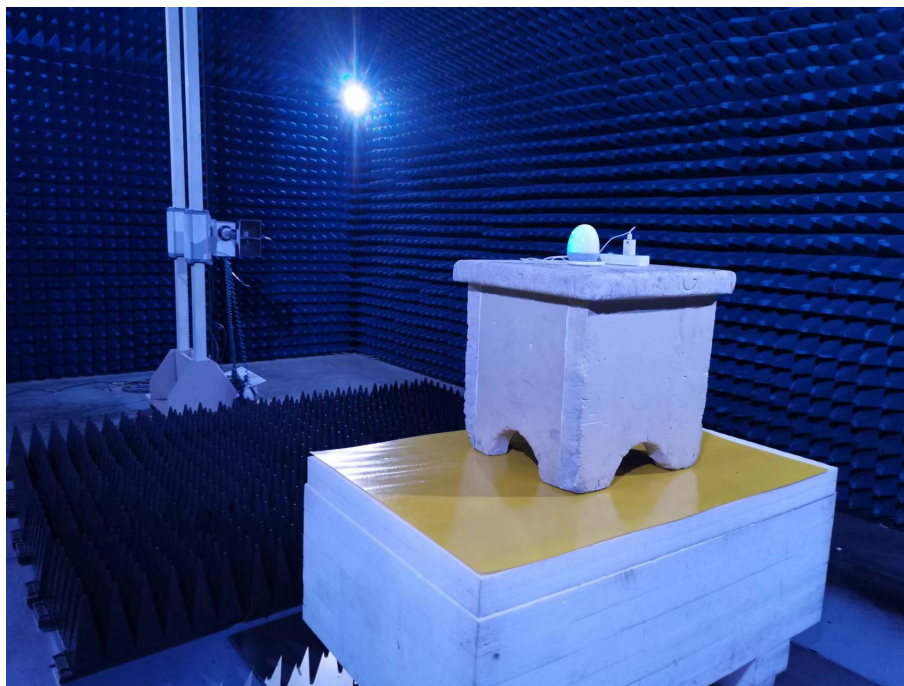
Photo of Radiated Emission Measurement (Above 1G)
