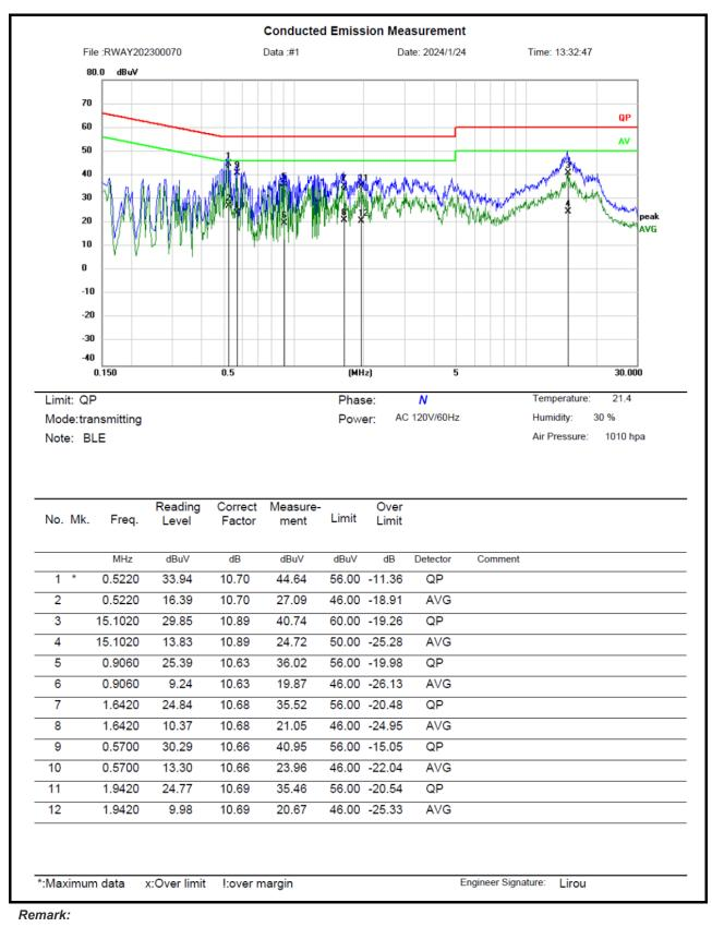
Measurement (dBuV)= Reading Level (dBuV) + Correct Factor(dB)
