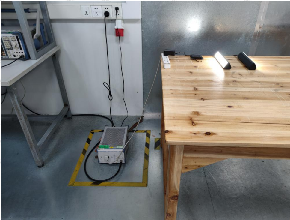
Photo of Conducted Emission Measurement
