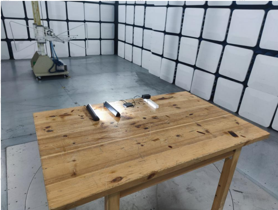
Photo of Radiation Emission Test
