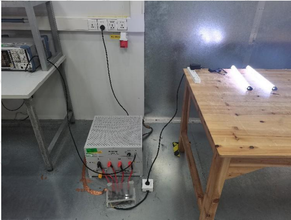
Photo of Conducted Emission Measurement
