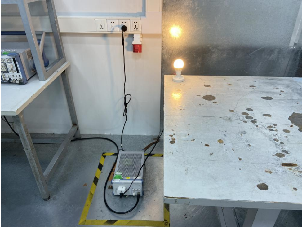
Photo of Conducted Emission Measurement
