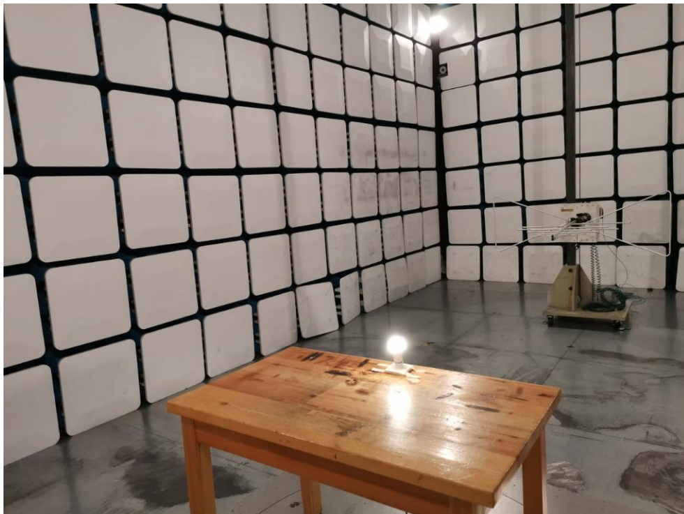
Photo of Radiation Emission Test
