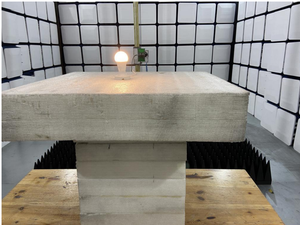
Photo of Radiation Emission Test
