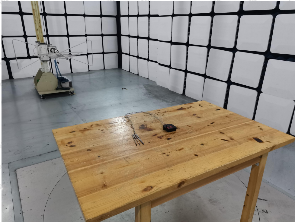
Photo of Radiation Emission Test
