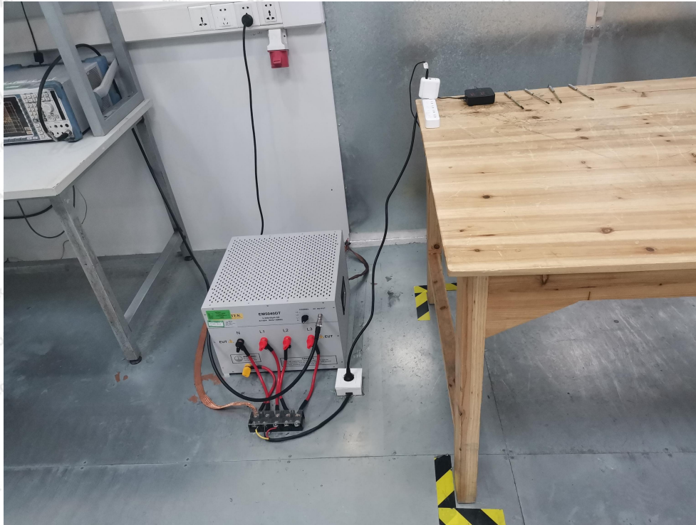
Photo of Conducted Emission Measurement
