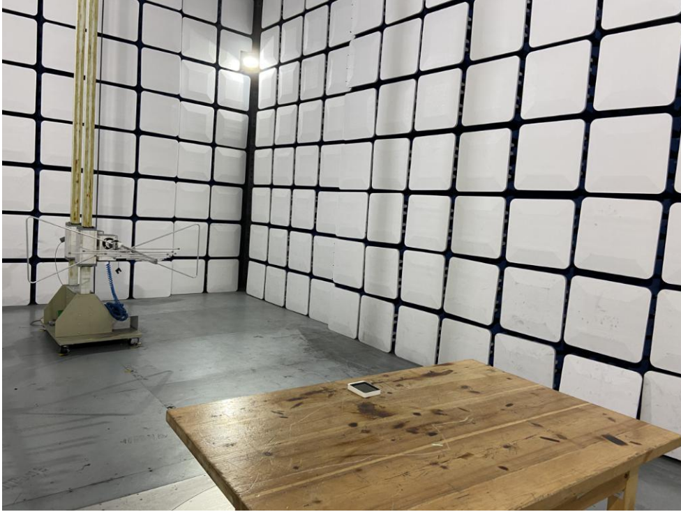
Photo of Radiation Emission Test
