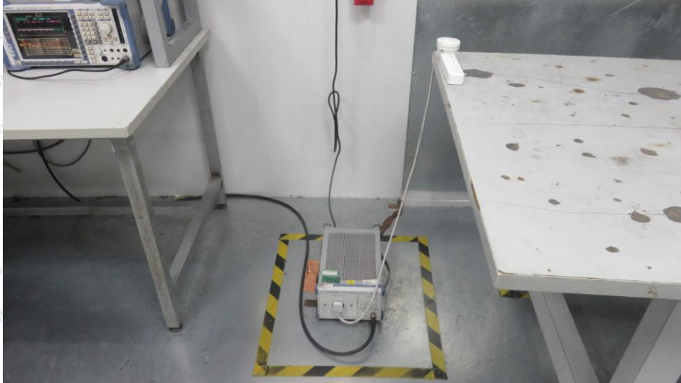
Photo of Conducted Emission Measurement
