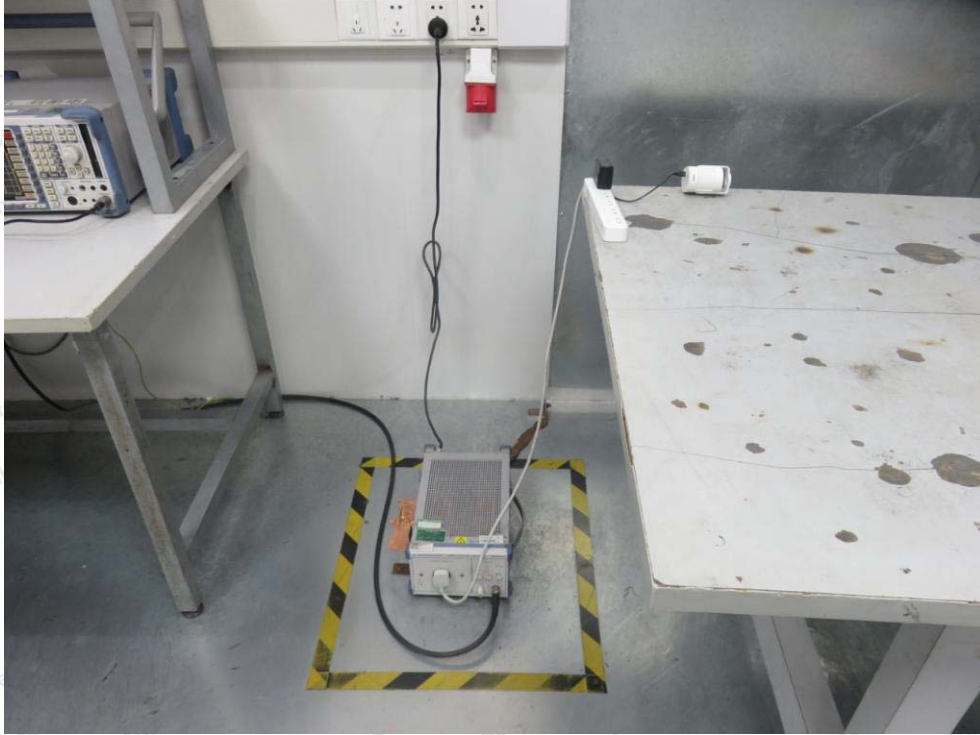
Photo of Power Line Conducted Emission Test
