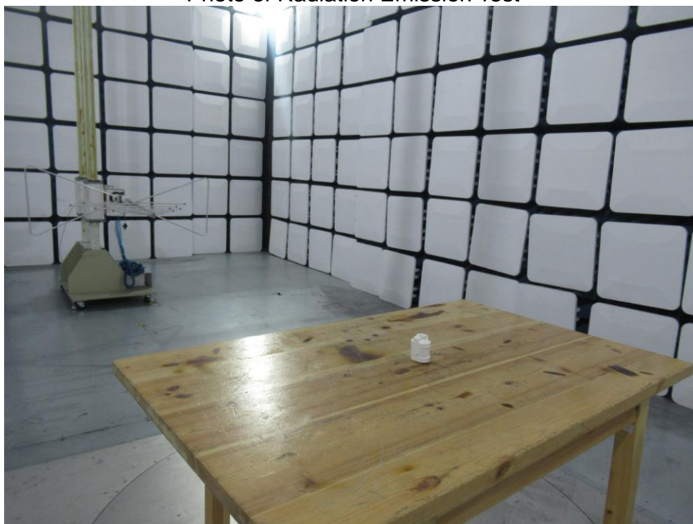
Photo of Radiation Emission Test
