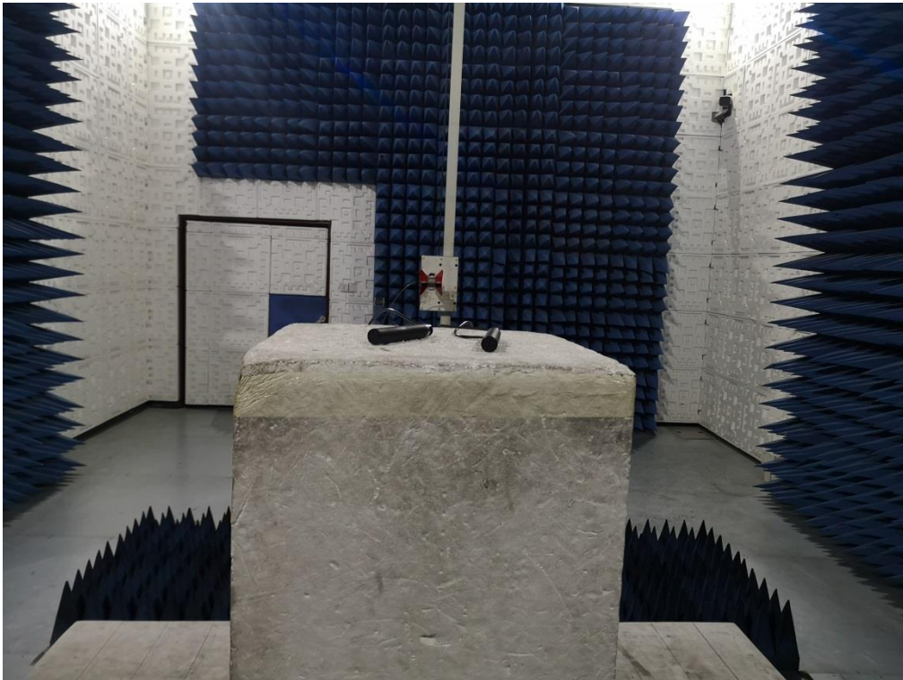
RADIATED EMISSION TEST SETUP ABOVE 1GHZ
