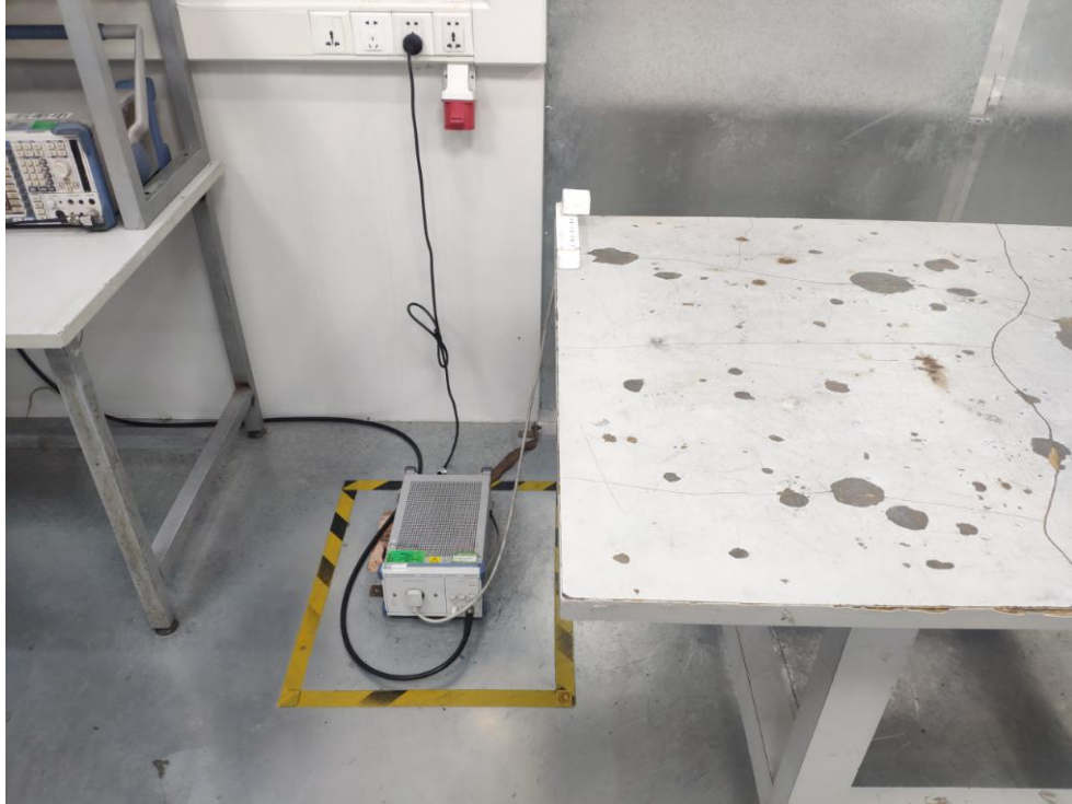
Photo of Power Line Conducted Emission Test
