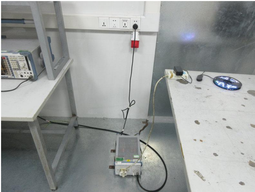
Photo of Power Line Conducted Emission Test
