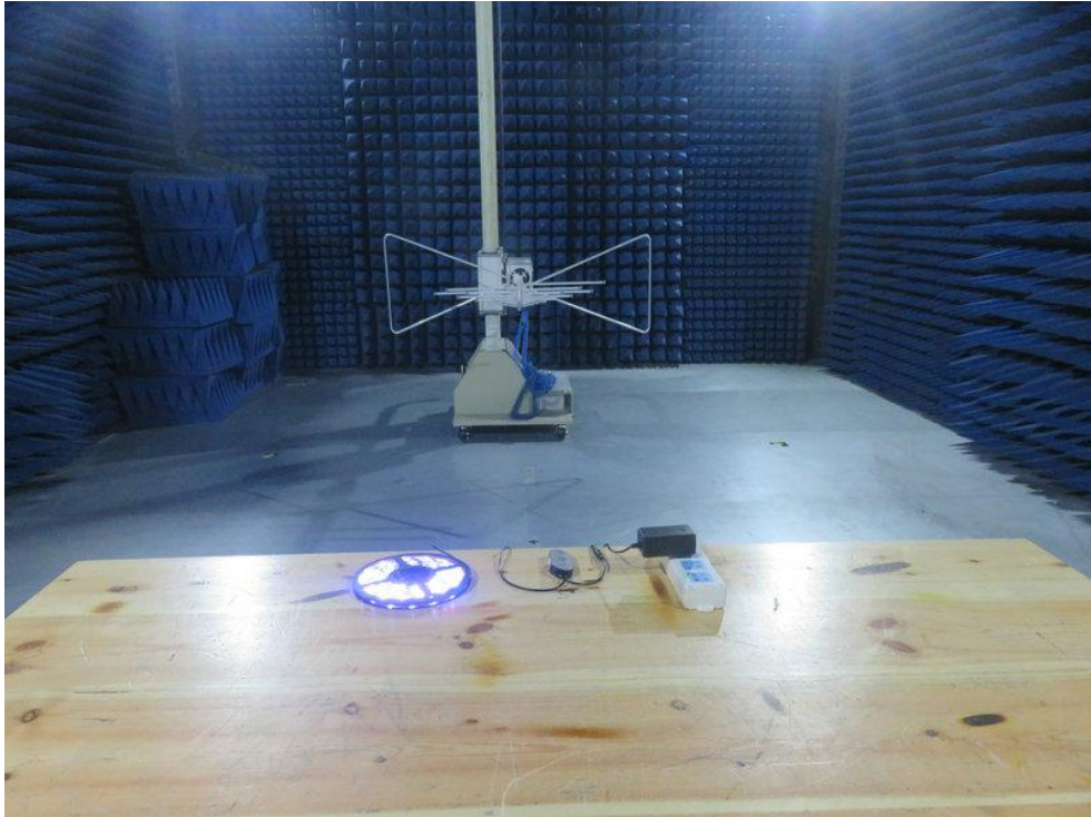
Photo of Radiation Emission Test
