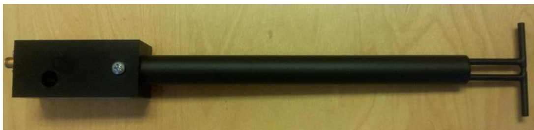
Figure 1 – MVG COMOSAR Validation Dipole
