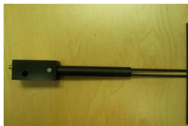
Figure 1 – MVG COMOSAR Validation Dipole
