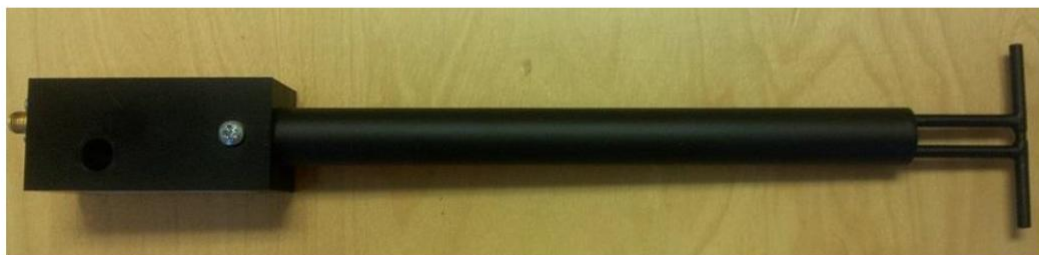
Figure 1 – MVG COMOSAR Validation Dipole
