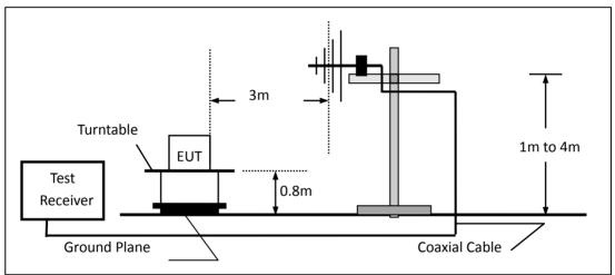
(c) For radiated emissions above 1000MHz
