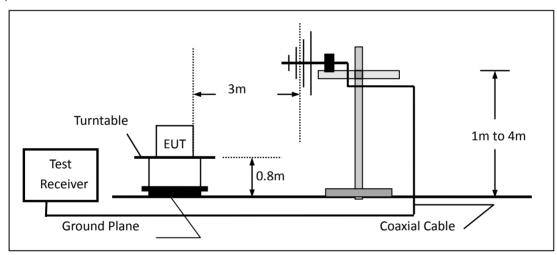
(c) For radiated emissions above 1000MHz
