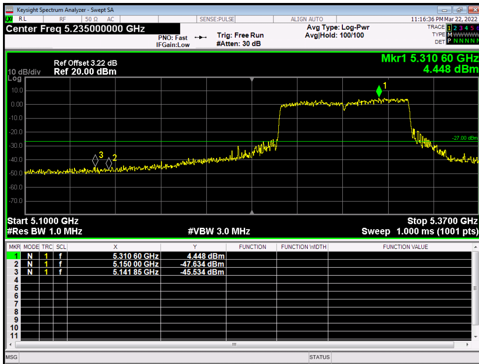
Band Edge NVNT n20 5260MHz Low Ant1
