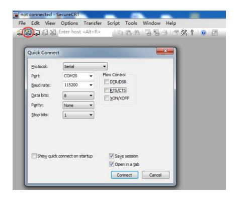
Among them, select Serial for Protocol, select COM port for computer identification of the module for Port, select 115200 for Baud rate, select 8 for Data bits, select None for Parity, select 1 for Stop bits, and uncheck any options in Flow Control. Then click Connect. After success, it is shown in the following figure:
