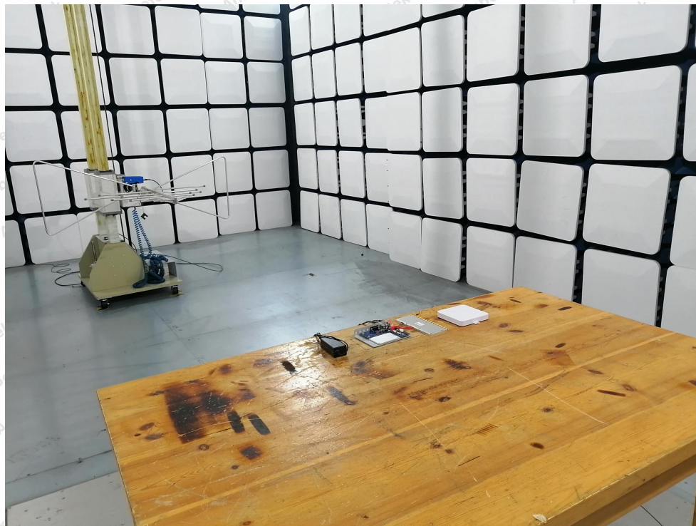
Photo of Radiation Emission Test
