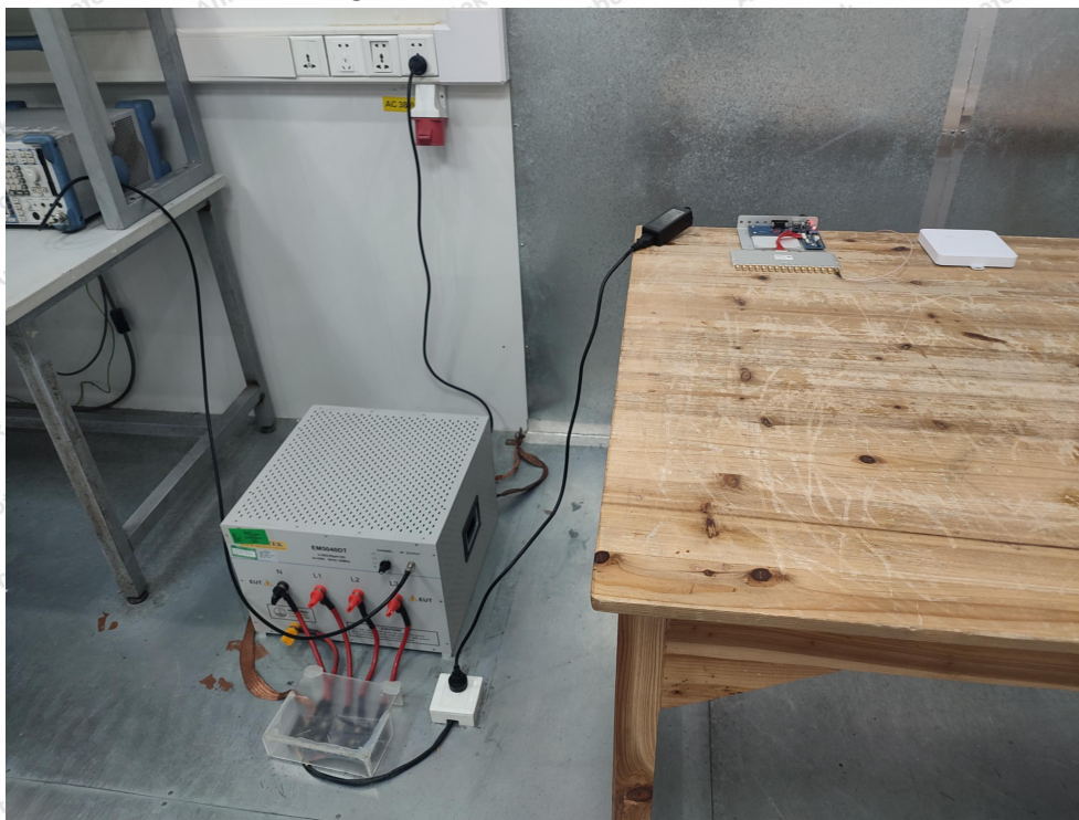
Photo of Conducted Emission Measurement
