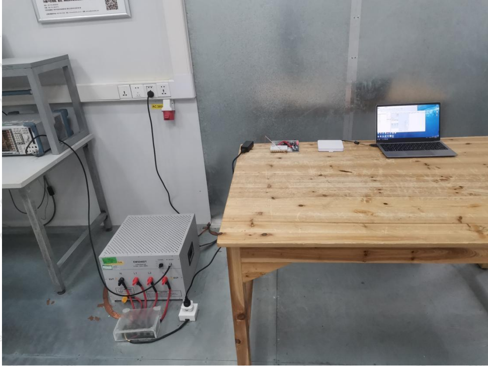
Photo of Conducted Emission Measurement
