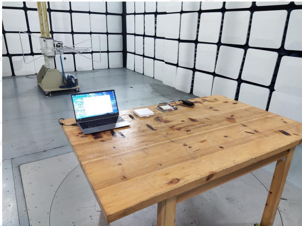
Photo of Radiation Emission Test
