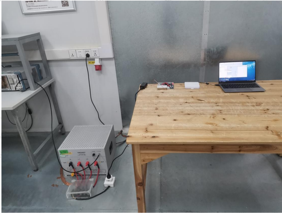
Photo of Conducted Emission Measurement
