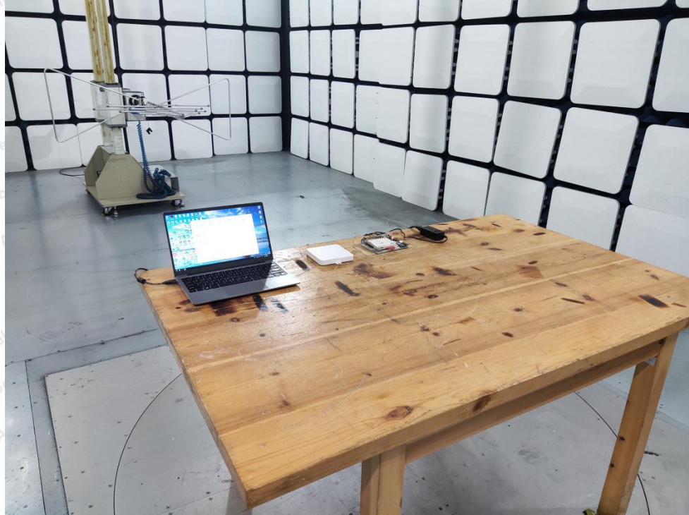
Photo of Radiation Emission Test
