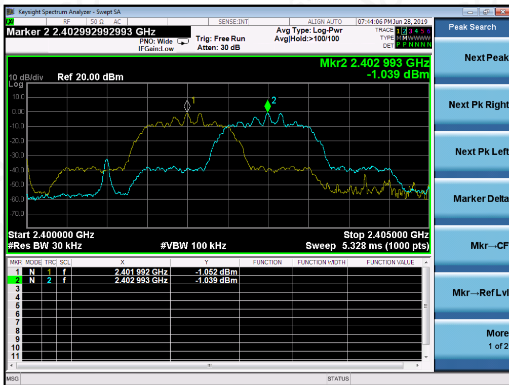
TEST PLOT FOR FREQUENCY SEPARATION
