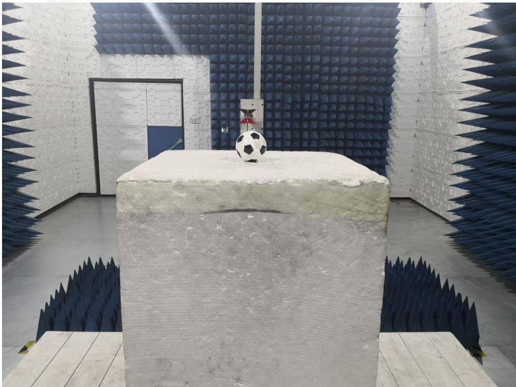
RADIATED EMISSION TEST SETUP ABOVE 1GHZ
