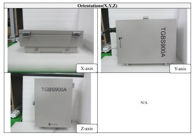
Note: Radiated testing was performed with the EUT in worst case X-axis.
