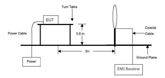
The diagram below shows the test setup that is utilized to make the measurements for emission from 30 Mz to 1 GHz emissions.
