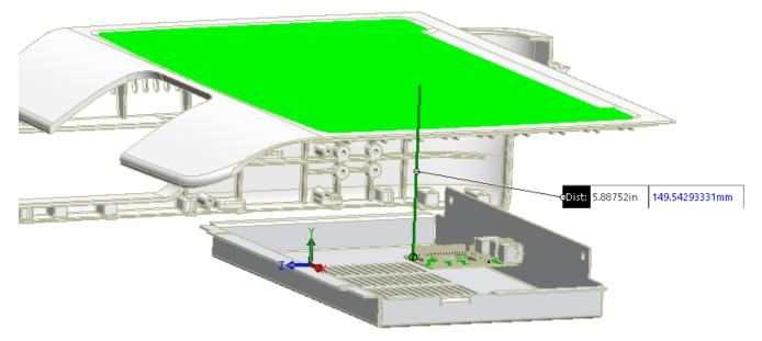
The closest exposure distance for the BLE external whip antenna occurs when a user places their hand on top of the work surface directly above the antenna. BLE external whip antenna is situated 13-25mm from the top cover.
