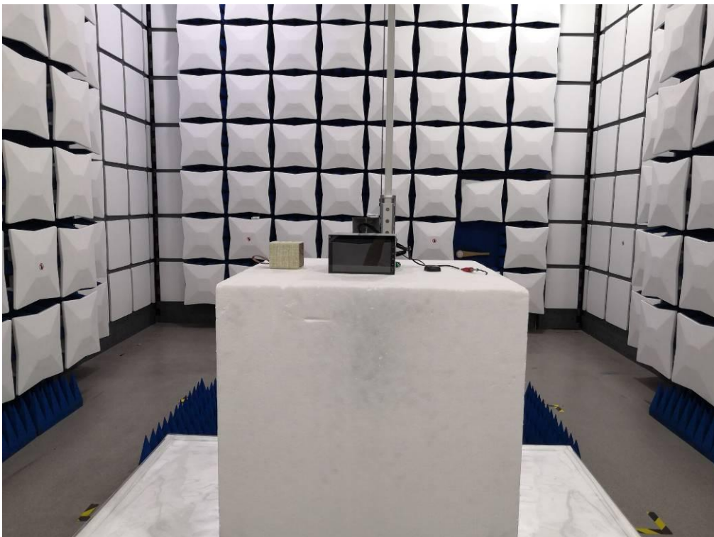
FCC RADIATED EMISSION TEST SETUP ABOVE 1GHZ
