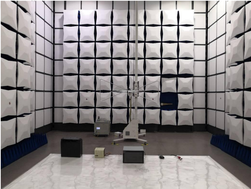
FCC RADIATED EMISSION TEST SETUP ABOVE 1GHZ
