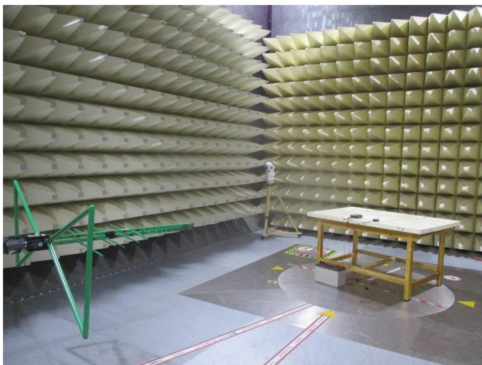
Photograph 2: Set-up photo for Radiated Emission, 30MHz - 1GHz
