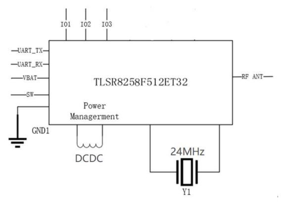
It embeds Flash, LDO and DCDC, crystal, RF match network and etc. With the high integration level of the module, few external components are needed to satisfy customers' ultra-low cost requirements.
